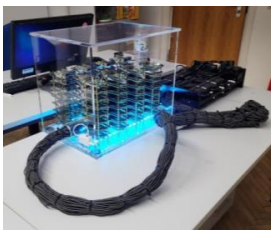
Fig. 1. Raspberry cluster (left) with service module (right)
